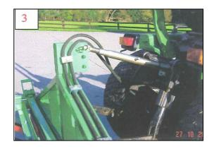
Raise the Sarel Roller to transport height using the tractor hydraulics.
