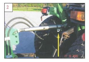
Fit the upper link (supplied with the Multi-Sarel). Ensure the upper spring anchor is at the tractor end of the link.
