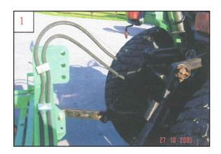
Fit the tractor lower link arms to the lower linkage pins with the tractor and secure with the lynch pins.
