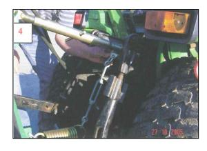
The flotation spring assembly can now be easily fitted to the upper spring anchor. Ensure the 'D' shackle is tightened securely.
