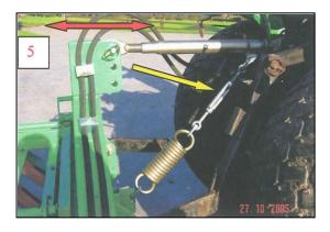
Ensure the Multi-Sarel parking stands are raised, then lower the it to the ground, and adjust the upper link to ensure the Multi-Sarel headstock is vertical. Open the wing sections and adjust the turnbuckle to obtain the required flotation of the main frame.
