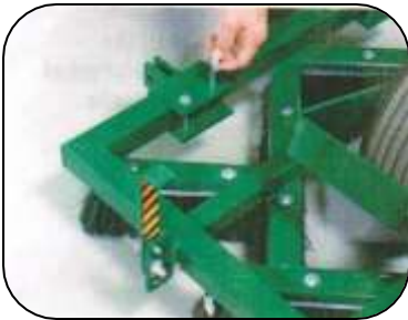
Attach extension wing brackets to the main frame of the Groomer. Do not tighten.
