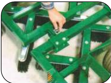
Attach each wing to the two extension wing brackets. Only tighten to a snug position so that the wings will fully rotate.
