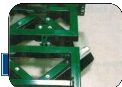
Align the frame of each wing with the frame of the Groomer. Fully tighten the two bolts of the extension wing brackets.
