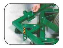
Attach extension wing brackets to the main frame of the Groomer. Do not tighten.
