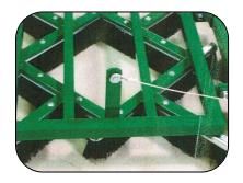
Attach the loose end of the cable to the upright arm of each wing.
