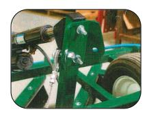
Attach the cable bracket to the upright arm of the wheel assembly on the Groomer. Attach one end of the cable to the bracket.
