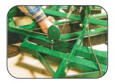
Attach the cable sheave bracket to the frame of the Groomer. The sheave bracket should be placed 26-1/2 inches from the outside of the Greens Groomer frame.
