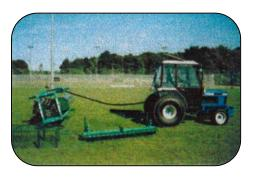
**9.** As soon as the Double-Quick starts to continue rolling under its own momentum STOP the tractor and allow it to come to rest on its 4 legs by itself.
