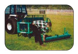
2. If a rear attachment is fitted, remove it by means of the 4 clevis pins and put it to one side.
