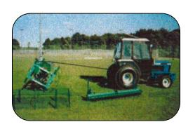
**8.** Ensure all bystanders keep back and drive the tractor very slowly forward causing the Double-Quick to rotate.
