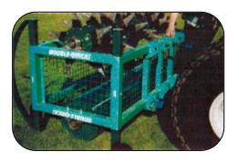
**10.** Reverse the tractor and re-attach the 3 point linkage.
