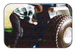
**6.** Attach the tow cable provided to the top link position on the tractor.
