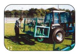
**12.** Raise the stand legs and lock up into the working position.
