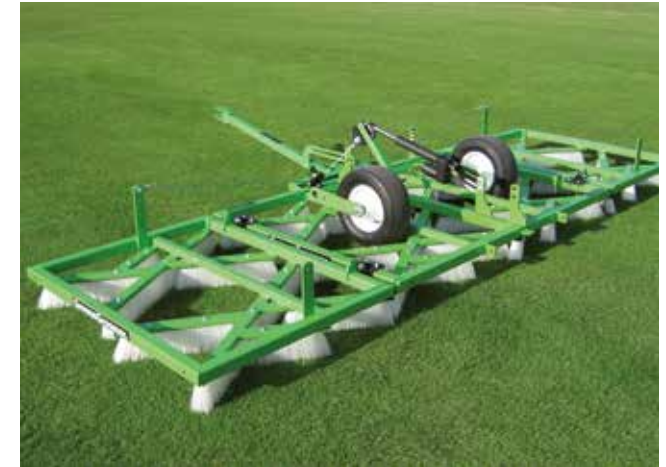
Full 12' (3.6m) working width with automatic folding wings.
