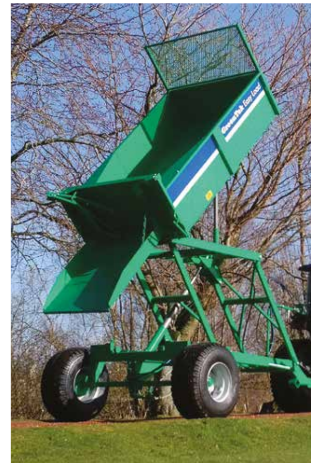
Wheels spaced outside body width provide extra stability for high tipping.
