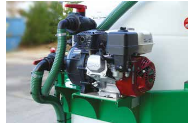
5hp Honda engine with high capacity pump
