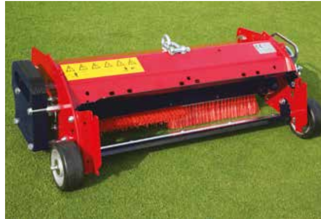
Contra-rotating brush units flick up aeration cores
