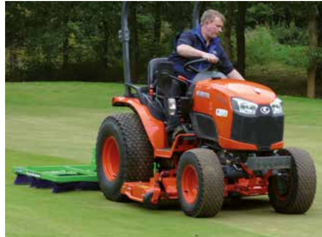
Brushes sand down coring holes
