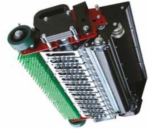
Seed is precisely metered out at the most economical application rate and pushed into the holes by the rotating spikes.
