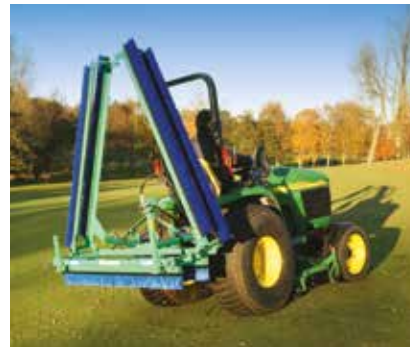
Hydraulic Maxi-Brush folds up without leaving your seat.
